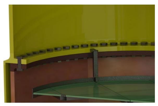
Figure 10-12. Bolted Connection Between the Transition Piece and Monopile Flange
