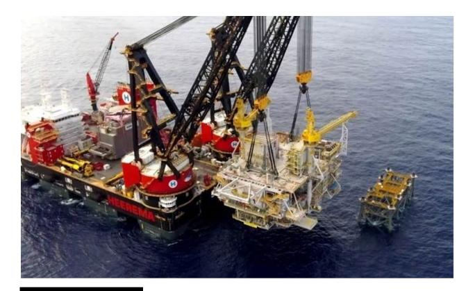
Figure 10-9. Heavy Lift Vessel for Installation of Offshore Converter Station
